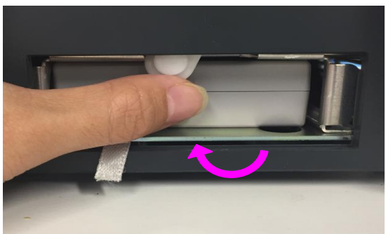
⑤ Turn the lever clockwise to keep the battery in place
