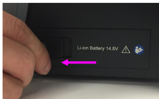
⑤ Replace the battery compartment door
