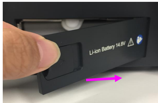
② Pull the battery compartment door out
