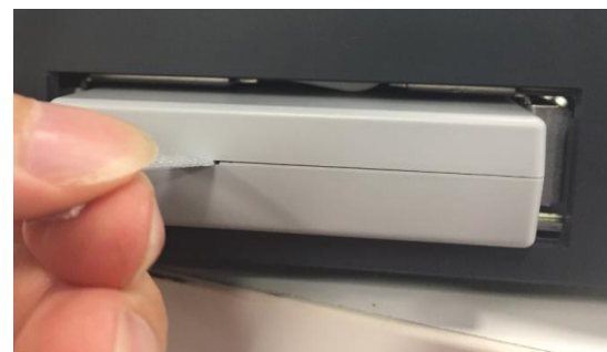
④ Pull the battery out
