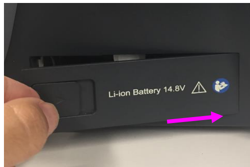
② Pull the battery compartment door out
