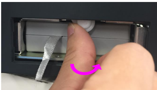
③ Turn the lever counter-clockwise to hide it
